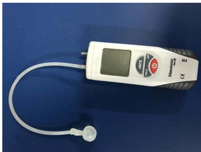
Fig. 4. Mechanical force measuring device, which is composed of a 0.5 cm silicone hollow sphere and a digital manometer.
